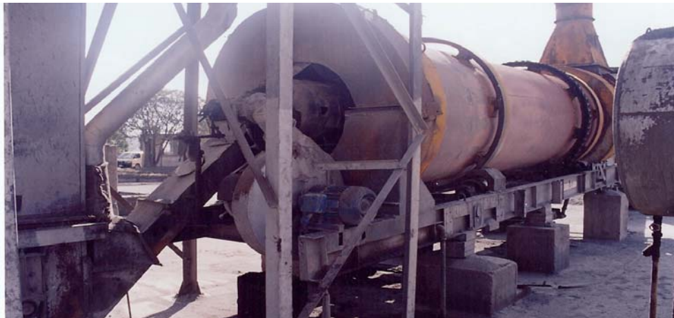
Asphalt Plant aggregate drum with no temperature gauge on Nanyuki Road, Industrial Area
